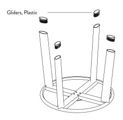
4. Remove the gliders with a flatheaded screwdriver.
