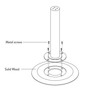
2. Screw counterclockwise to loosen the seat from the rod.
